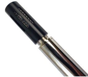
Figure 1 - Remove protective cap from the T/H Probe turning counterclockwise.
