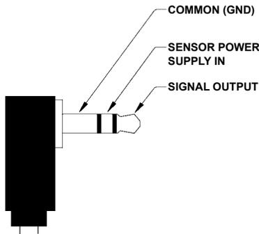
RCA Output Connector - Connection Detail
