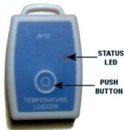
The logger has a bi-colored LED that is used to indicate record status and alarms when the button is pressed momentarily. The LED blinks twice – the first blink is the Record status and the second blink is the alarm status. The button can also be used to stop and start the recording if programmed by the user.
