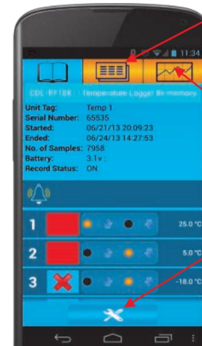
Touching the data tab will initiate a full data download. Place Logger in NFC antenna location and hold in place. Full data transfer can take up to 8 seconds.
