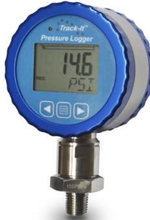
Data Loggers can be ordered in various ranges (see back for details). The logger is packaged in a rugged submersible anodized aluminum and stainless steel housing and has a standard 1/4" NPT fitting (1/2" NPT for 8700 and 14500 ranges). The replaceable internal lithium battery has up to a 3-year life.
