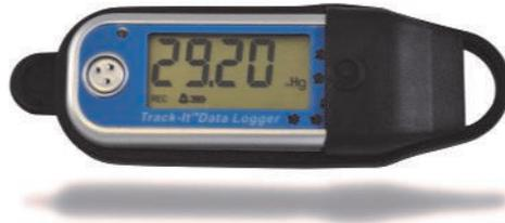
user selectable and can be sequenced by pressing the logger button. There is a multicolored LED indicator to notify user of alarms or general activity. A splash proof protective cover protects the logger when in use. Additionally, the logger can be used to record external inputs using optional Track-It DC voltage or DC current modules.
