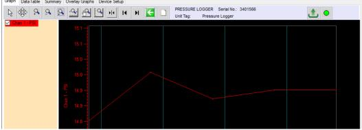
Clear the logger and start a new recording by clicking the Device Setup Tab, then Send Config.
