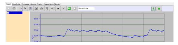
Clear the Data Logger and start a new record by clicking the Device Setup Tab, then Send Config.
