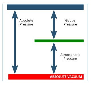
Track-It pressure loggers with PSIA sensors will indicate approximately 14.7 PSI at sea level when the pressure port is open to atmosphere (i.e., sitting on a desk or bench during set up). This reading will fluctuate slightly with atmospheric pressure changes and will be more noticeable on sensors with smaller pressure ranges.
